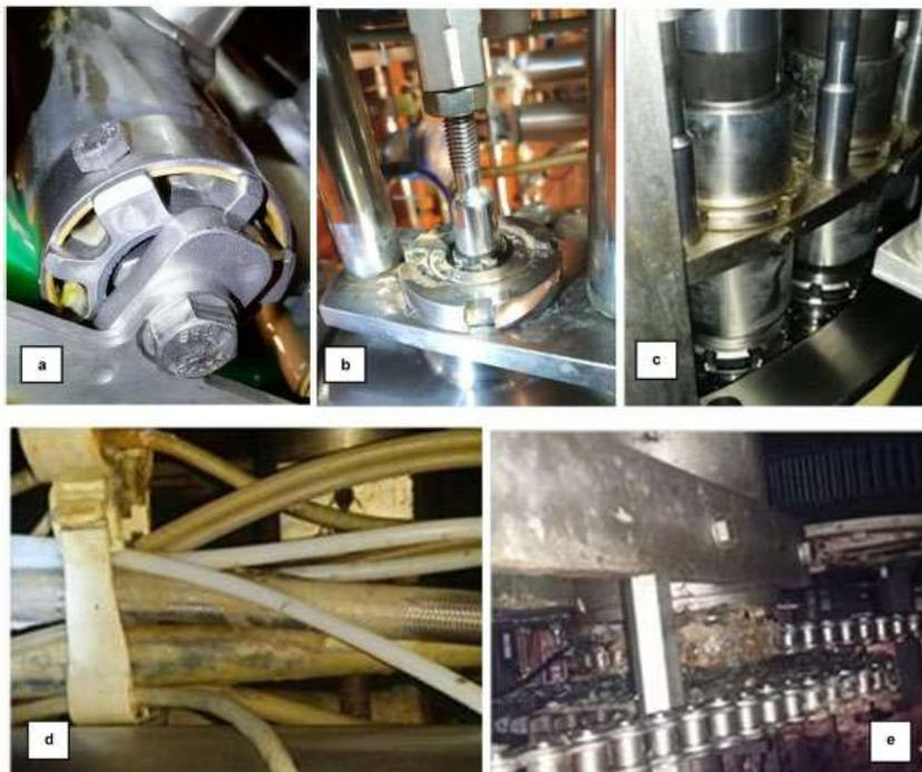
Fig. 2. Brewery points where biofilms with *Pectinatus* were detected: bottle raising pistons in filler (a); entry beer modulating valve (b); bottle raising pistons in crowner (c); bundles of cable lines (d); transmission chains (e).
